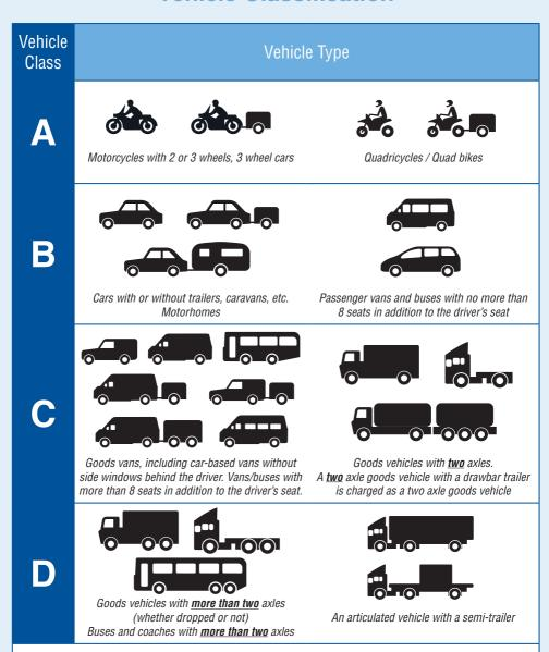
The number of axles includes drop axles, whether they are up or down. Trailer axles are not included but articulated vehicles include all axles including attached semi-trailer axles.
